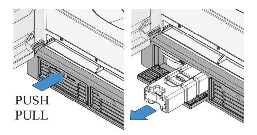
• remove the protective cover from the new filter;
