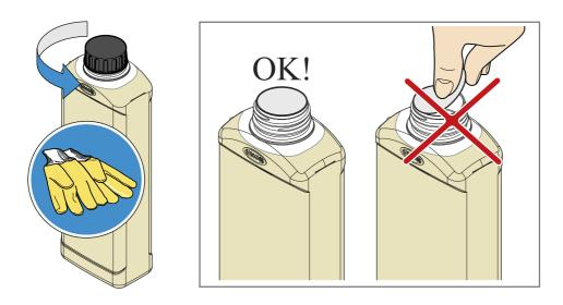
check that the protective film is intact and undamaged. Turn the bottle upside down and screw it onto the tank; a pin will break the protective film, which allows the detergent to pass safely into the tank.
