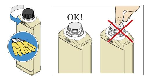
• check that the protective film is intact and undamaged. Turn the bottle upside down and screw it onto the tank; a pin will break the protective film, which allows the detergent to pass safely into the tank.
