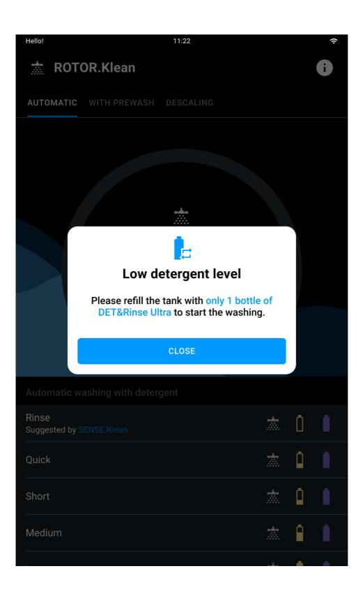
You must only refill the tank with 1 litre | 0.26 US Gal bottles of UNOX Det&Rinse<sup>™</sup> Ultra detergent, the only one approved and tested for washing the oven cavity.
