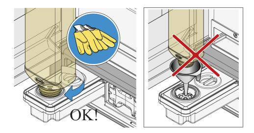
• When the bottle is completely empty, remove it, making sure it doesn't drip; dispose of it as prescribed by current regulations.
