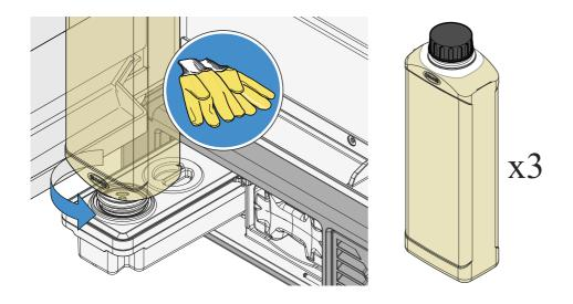
Repeat the process until the tank's maximum capacity is reached (3 litres | 0.79 US Gal= 3 bottles of UNOX Det&Rinse<sup>™</sup> Ultra), then put the tank back in until it can go no further. Dispose of the gloves without touching the areas wet with detergent.
