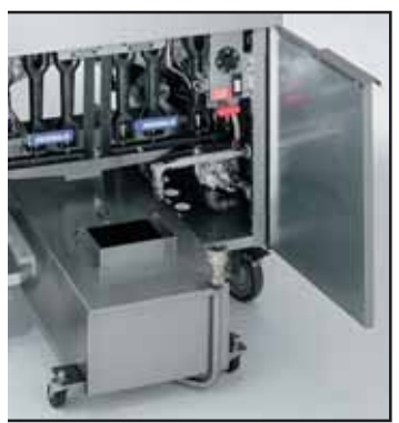
Fryer Filter System Filtering system is conveniently under the fryers to save space. A roller pump speeds the process to save time. The oversized 4" square manifold is clog free.
