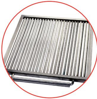
FLOATING ROD, STEEL STANDARD TOP GRIDS Cold-rolled steel or chrome plated. Standard Spacing 5/16" Between Rods Fish Spacing 3/16" between rods
