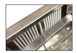
**ADJUSTABLE TRAY PLATFORM...**Field adjustable springs to accommodate differences in tray weights and heights. Number of connected springs can be increased or decreased to change the platform tension.
