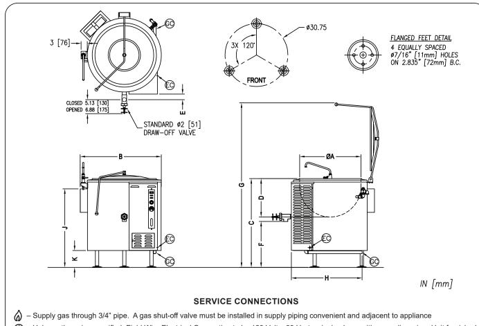
(F) – Unless other wise specified, Field Wire Electrical Connection to be 120 Volts, 60 Hertz, single phase with grounding wire. Unit furnished with 6' cord and 3 prong plug. Total maximum amps 4.0.
