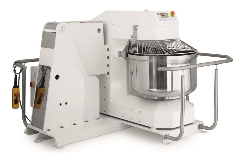
Spiral Mixer, 280 Lb. Dough Capacity, 2 Speeds, Programmable Digital Control, Stationary Stainless Steel Bowl, Safety Guard & Dough Hook, Cast Iron Frame with Enamel Coated Steel Finish, 2 HP Hydraulic Lift, Protective Rail Dropping at 57 1/8", 2 HP Bowl & 10 HP Hook, 208-240V/60/3P/32A, NEMA 15-50P
