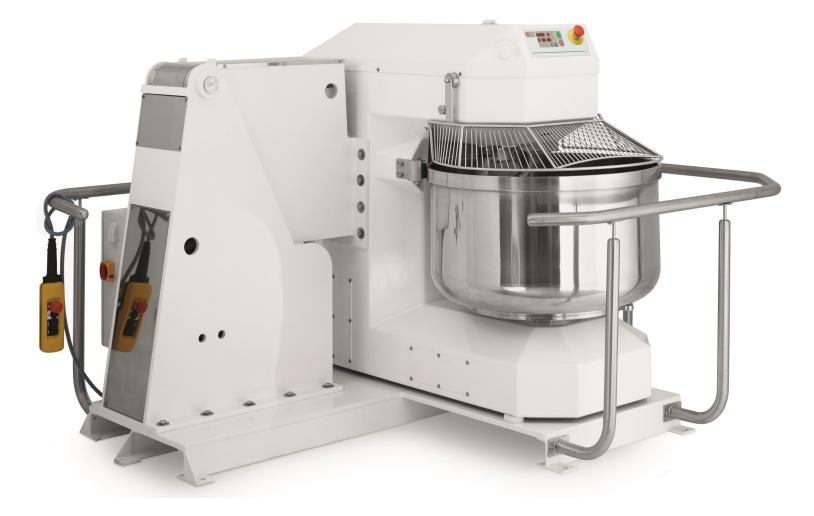
Spiral Mixer, 520 Lb. Dough Capacity, 2 Speeds, Programmable Digital Control, Stationary Stainless Steel Bowl, Safety Guard & Dough Hook, Cast Iron Frame with Enamel Coated Steel Finish, Protective Rail Dropping at 53 5/8", 10 & 2 HP (Hook & Bowl), 208-240/60/3P/32A, NEMA 15-30P
