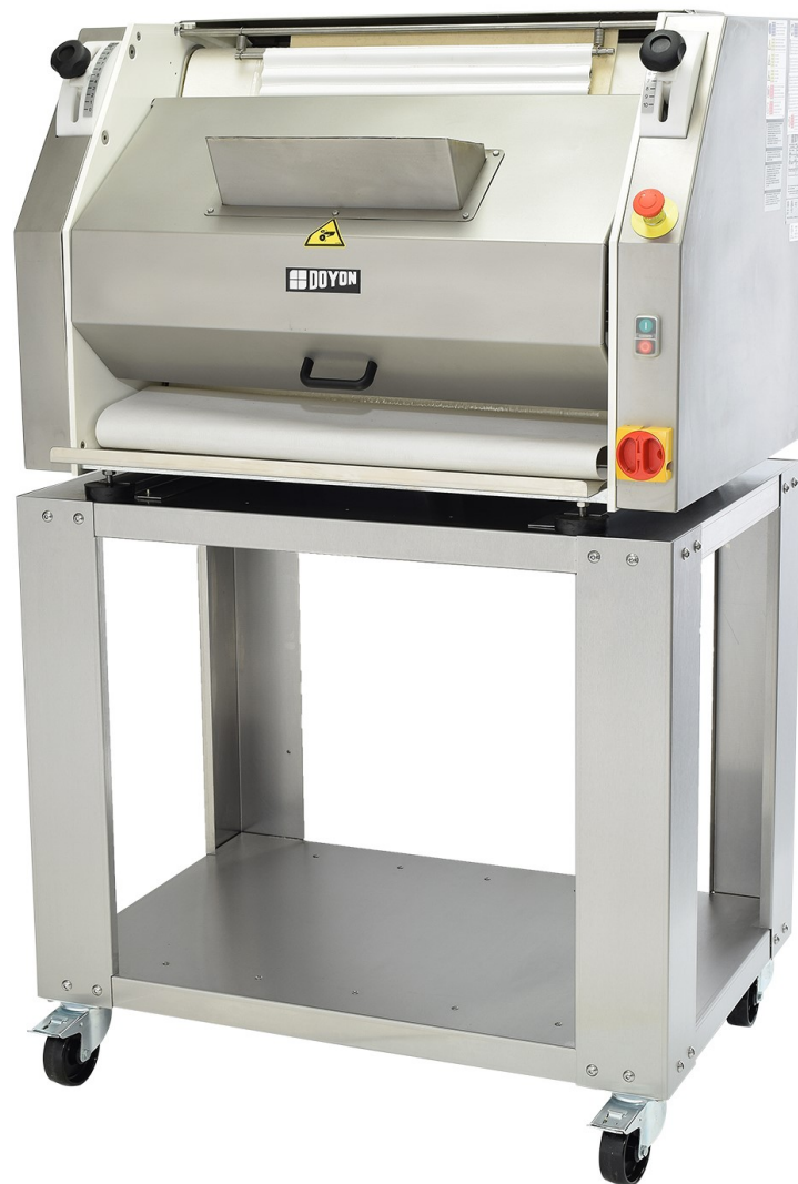
Automatic Dough Moulder, 3 Roller Infeed, Stainless Steel Construction, Hopper Safety System, Synthetic Belt, Retractable Outfeed Table, 1 1/2 HP, Production Up to 2500 Pieces/Hour
