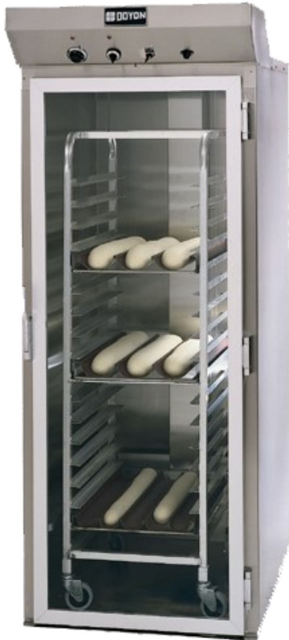
Proofer Cabinet, Roll-In, One-Cavity, Single (1) Rack Capacity or (36) 18"x26" Sheet Pans, Solid State Heat & Humidity Controls, Auto Water Entry, Full View Glass Door, Stainless Steel Interior and Exterior, Aluminum Floor, NSF, cETLus, ETL
