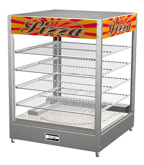
Food Warmer/Display Case, Countertop, Four Shelf Interior Rack, Capacity (4) 18" Pizzas, Inside Water Pan for Humidity, Adjustable Heat Control, Tempered Glass Front, Sides & Door, Stainless Steel Construction, 120V/60/1P/11A
