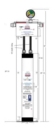
All IcePro cartridges should be changed out every six months or when there is a reduction in water pressure. Filter life depends greatly upon the quality of water. This product is for commercial use only and must be installed and maintained according to manufacturers guidelines www.icetroamerica.com or the warranty can be voided.
