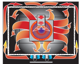
Convection oven cooks faster with less shrinkage.
