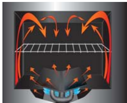
Linear burner for even heating throughout the oven cavity.
