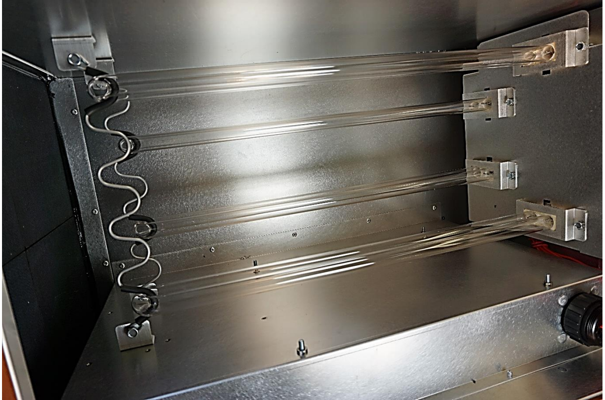
Figure 14: Completed Bulb Assembly
