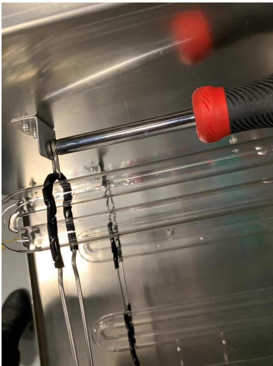
Figure 16: Install Bulb Support Wires
