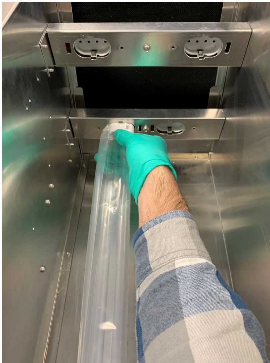
Figure 14: Install 4 New Bulbs. Do not Touch Bulbs with Bare Hands
