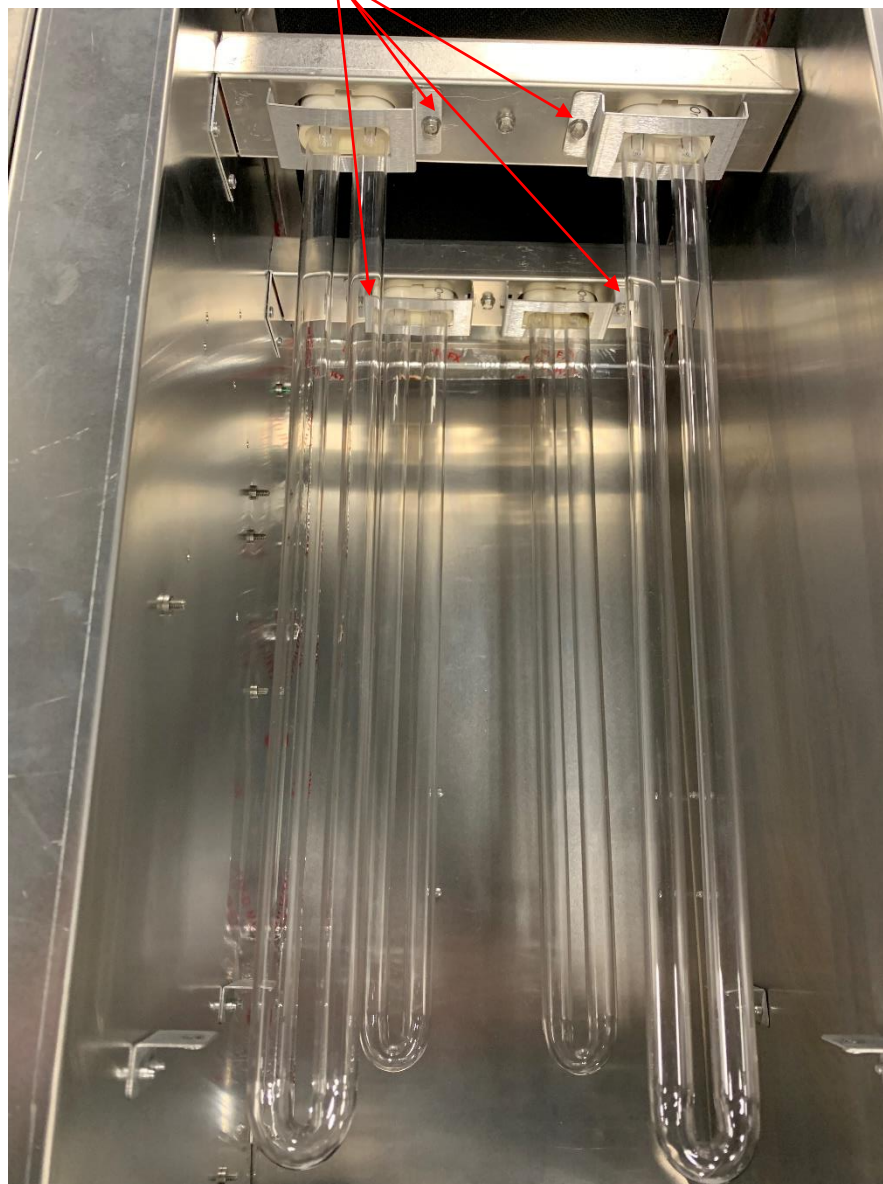
Figure 11: Remove 1/4" Screws on Bulb Support Clips
