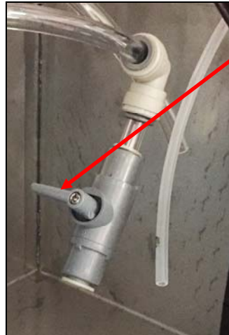
Fig. 2 Priming valve in OPEN position
