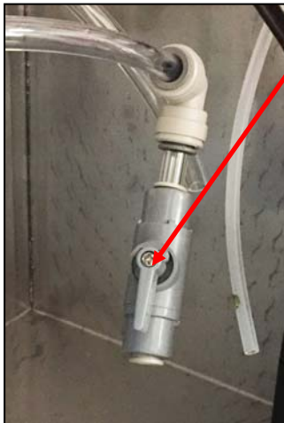
Fig. 2 Priming valve in OPEN position
