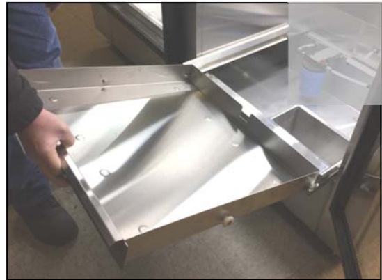
Fig. 1: Access the water reservoir
