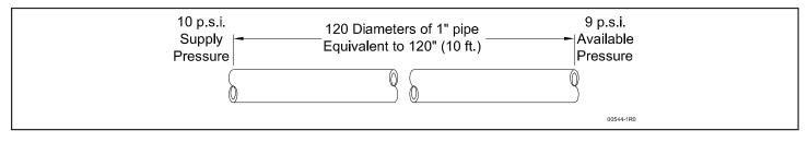
**NOTE**: In 3/4" pipe size, that a Standard 90° Elbow and Angle Valve and a Globe Valve are equivalent to 1.8 feet, 10 feet and 18 feet respectively of straight pipe.
