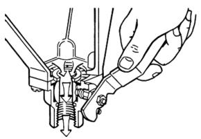
The Boiler Water Level Control installed on your boiler requires periodic maintenance. As boiler water circulates into the float chamber, sand, scale and other sediment may be deposited in the float chamber. While the chamber has been designed with a large accumulation bowl, it is necessary to flush the sediment from the chamber by blowing down the control so that the accumulation of sediment does not interfere with the movement of the float in the control.
