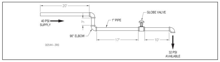
Total of above = 20 + 2.2 + 3 + 2.2 + 17 + 23 + 10 + 2.2 = 79.6 feet. Since each 10 feet is equivalent to 1 psi pressure loss, 79.6 feet is equivalent to approximately 32 psi from an original Boiler supply of 40 psi.
