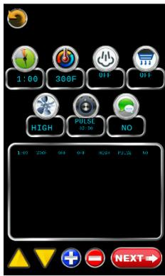
You can select off, on, pulse or delay vent. If you select on it will be on for the entire stage. If you select pulse it will come on and off with the time entered. If you select delay it will come on after the delay time entered and stay on for the on time entered. After the changes are made touch
