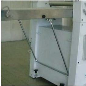
Fig. 3.1 Fig. 3.2 Also, lower the security bars (fig. 3.3 and 3.4) near the canvas.
