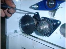
10. Remove the conveyor belt rollers.
