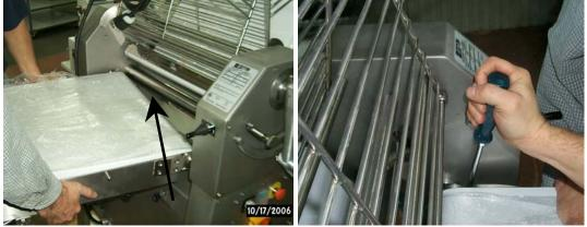
In same time you push the spring load, insert the opposite side of the conveyor in the front slut.
