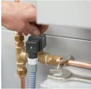
Fig. 7.3 Loosen the nut against the solenoid.
