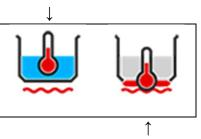
Right icon: secondary control (when the SETPOINT is reached, the heating stops)
