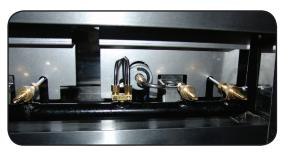
2. Unscrew bolts and pilot valve, then remove the manifold.
