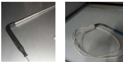
Figure 2: NTC Needle Probe Types
