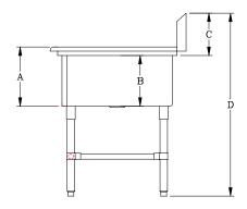
All dimensions are typical. Tolerance +/- .500". All units ship unassembled for reduced shipping cost.
