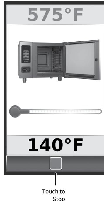
The target oven temperature chosen will appear just above the red Stop button.
