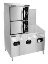
The CSD-1 compliant steam generator comes standard with a Pilotless Ignition System and Nickel Plating. The steam generator will be automatically filled with water and brought to pressure when water and heat switches are turned on and automatically drained under pressure when water and heat switches are turned off. A cold water condenser will automatically condense all exhausted steam into water before it is released from the cooker and steam generator drain.
