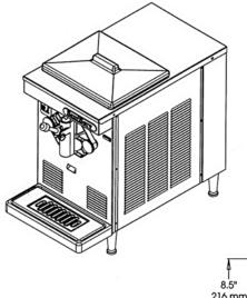
Minimum Wall Clearance Both Sides and Back -6 inches (152 mm)
