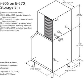
Space-Saving Designs i-906 i-906 B-570 B-970\* 76.50" Height 76.50" 194.30 cm 194.30 cm Width 30.00" 48.00" 76.20 cm 121.92 cm 34.00" 34.00" Depth 86.30 cm 86.30 cm 430 lbs. 710 lbs. Bin Storage 195 kgs. 322.2 kgs. Height includes adjustable bin legs 6.00" to 8.00", (15.24 to
