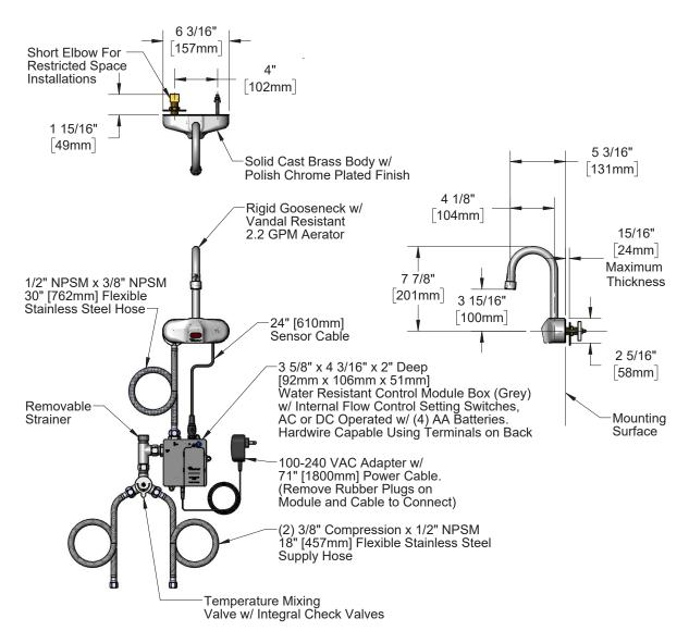
Rough-In Requirement: (2) 1" [25mm] Mounting Holes on 4" [102mm] Centers
