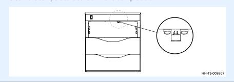
2. Suspend a multimeter thermocouple in the center of the drawer. Do not allow the thermocouple to touch any surface.
