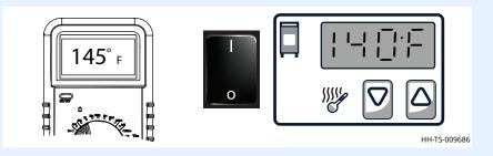
5. If the multimeter temperature and the Actual temperature don't match, **press** and **hold** the Up and down arrow buttons (2) for eight (8) seconds. The control will display the previous calibration offset value or 0.
