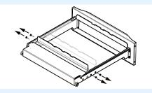
3. **Slide** the bracket to the back two (2) holes.
