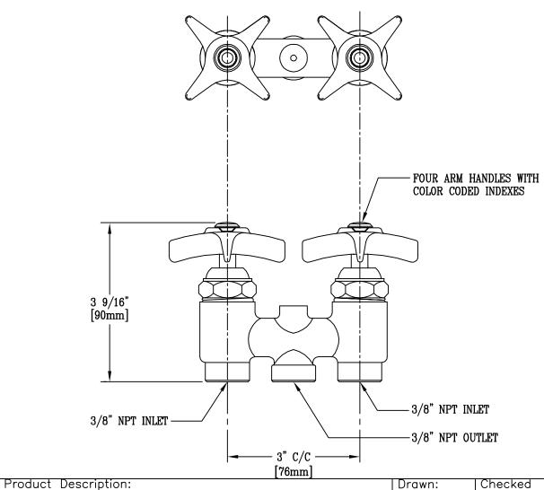
MIXING VALVE WITH 4-ARM HANDLES, 3" INLET CENTERS, AND 3/8" NPT
