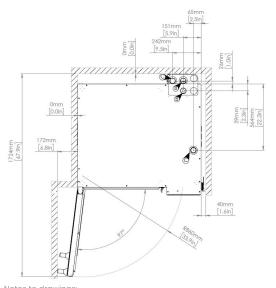
Notes to drawings: 400 mm / 15.75 inches spacing on right side of oven recommended for service access.
