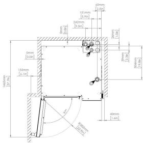
Notes to drawings: 400 mm / 15.75 inches spacing on right side of oven recommended for service access.
