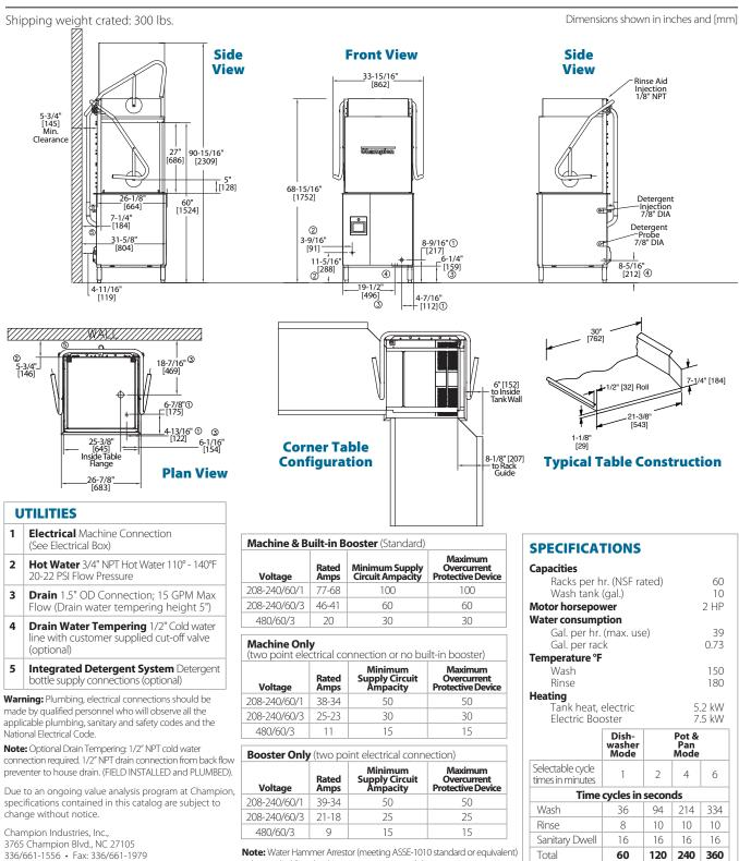
Note: Water Hammer Arrestor (meeting ASSE-1010 standard or equivaler to be supplied (by others) in common water supply line at service connection.
