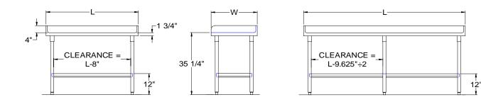
All units ship unassembled for reduced shipping cost. Units 7 ft. and larger are furnished with six legs. All dimensions are typical. Tolerance +/- .500".
