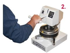
Set desired time. After heat indicating light has gone out, pull down the handle. When timer sounds, pull up the handle.
