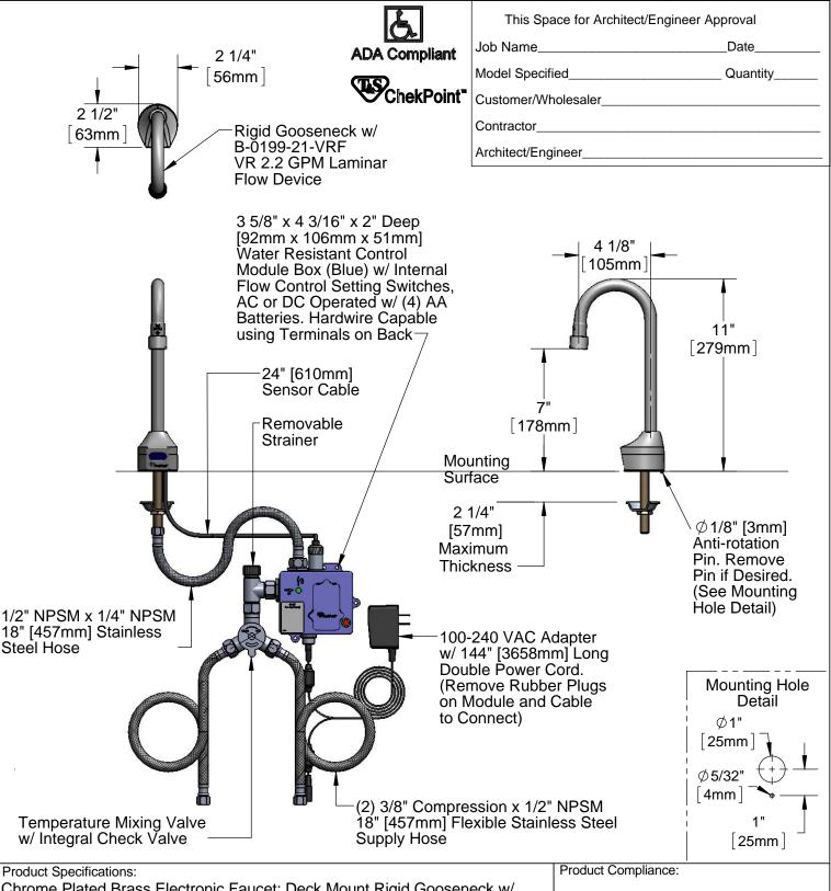
Chrome Plated Brass Electronic Faucet: Deck Mount Rigid Gooseneck w/ VR 2.2 GPM Laminar Flow Device, AC/DC Control Module w/ Internal Flow Control Setting Switches, Temperature Control Mixing Valve w/ Integral CheckValves, 18" Flexible Stainless Steel Supply Hoses
