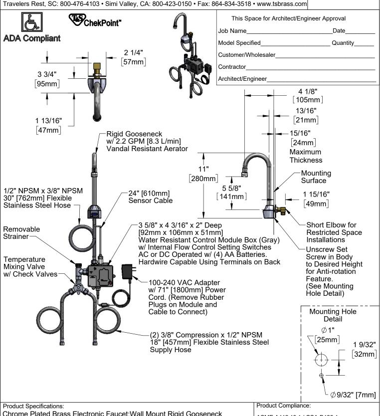
Chrome Plated Brass Electronic Faucet:Wall Mount Rigid Gooseneck w/ VR Aerator, AC/DC Control Module w/ Internal Flow Control Setting Switches, Temperature Control Mixing Valve w/ Check Valves, 18" Hot & Cold Supply Stop Flexible Connector Hoses
