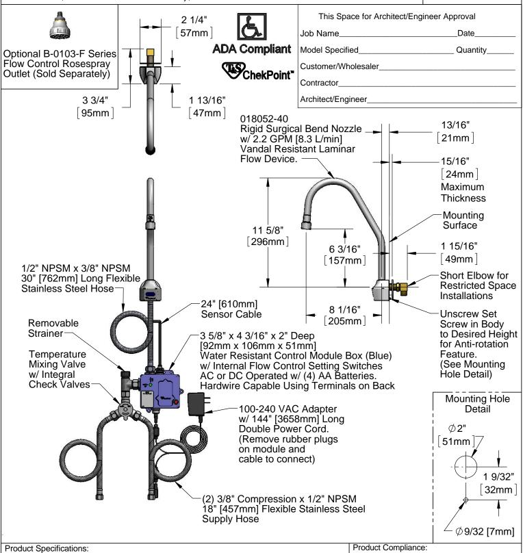
Chrome Plated Brass Electronic Faucet: Wall Mount Rigid Surgical Bend Nozzle w/ VR Laminar Flow Device, AC/DC Control Module w/ Internal Flow Control Setting Switches, Temperature Control Mixing Valve w/ Integral Check Valves, & 18" Lg Hot & Cold Supply Hoses
