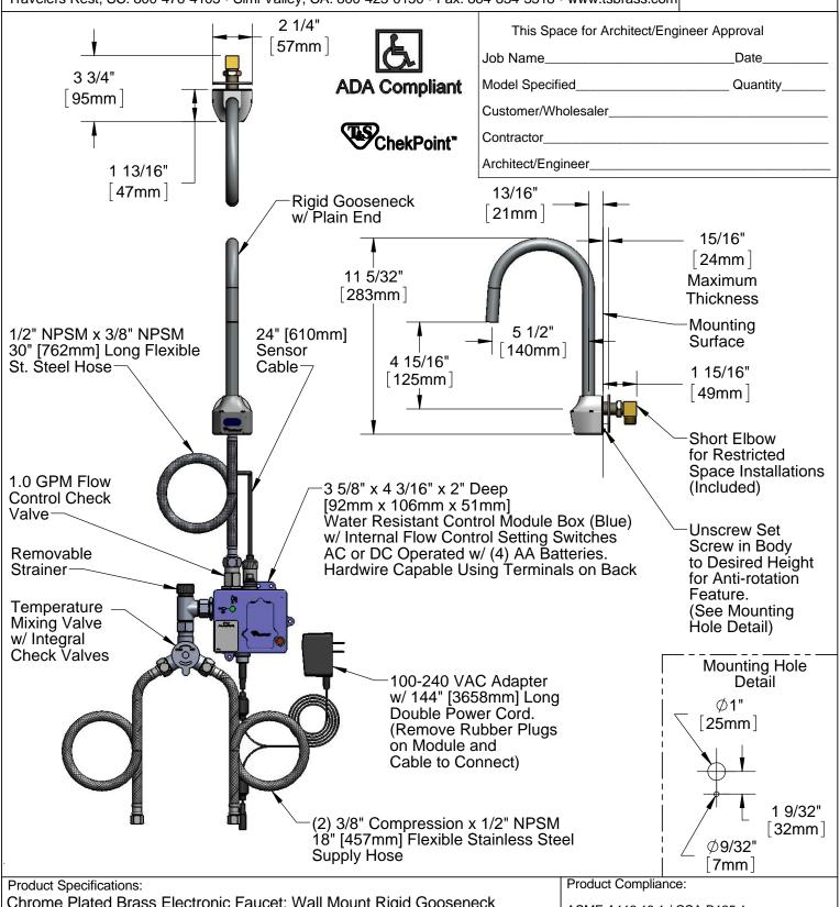
Chrome Plated Brass Electronic Faucet: Wall Mount Rigid Gooseneck w/ Plain End, AC/DC Cont. Module w/ Internal Flow Control Setting Switches, 1.0 GPM Flow Control Check Valve, Temperature Control Mixing Valve w/ Integral Check Valve, 18" Lg Hot & Cold Supply Stop Flexible Connector Hoses
