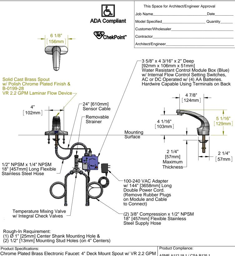
Chrome Plated Brass Electronic Faucet: 4" Deck Mount Spout w/ VR 2.2 GPN Laminar Flow Device, AC/DC Control Module w/ Internal Flow Control Setting Switches, Temperature Control Mixing Valve w/ Integral Check Valves, 18" Flexible Stainless Steel Supply Hoses
