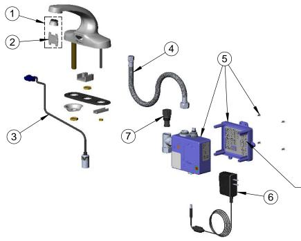
A Maximum of (8) ChekPoint Faucets can be Hardwire Connected and Powered by EC-HARDWIRE ChekPoint Hardwire AC Transformer. (Sold Separately)
