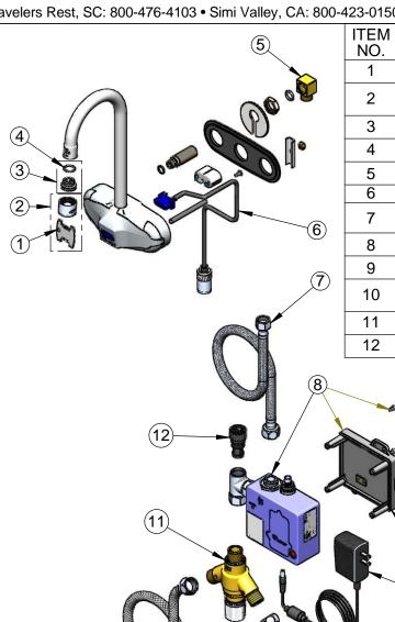
DESCRIPTION SALES NO. 015425-45 Vandal Resistant Key 0.5 GPM VR Non-Aerated Spray B-0199-06-N05 Device, 55/64-27 Female 3/8" to Aerator Adapter 044A 006575-45 -015 O-Ring Low Profile Elbow, 3/8 NPSM 015345-45 Angled Sensor with Cable 017195-45 Inlet Hose, Faucet, 1/2" NPSM-F x 3/8" 016325-45 NPSM-F ChekPoint Control Module 016647-45 5EF-0002 A/C Transformer Supply Hose, 9/16-24 Female x 1/2" 5EF-0005 NPSM EC-TMV ASSE 1070 Thermostatic Mixing Valve **EC-FILTER** Replacement Filter
