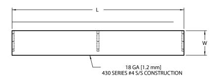
NOTE: BRACKETS SHIP LOOSE SHELF ATTACHES TO BRACKETS WITH SILICONE OR CONSTRUCTION ADHESIVE
