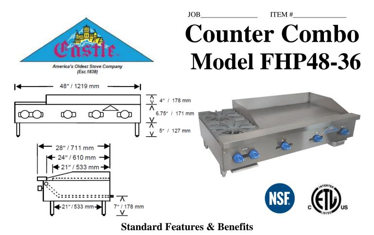
**CONSTRUCTION:** Easy cleaning, corrosion resistant stainless steel finish, welded with angle iron and aluminized inner framing. Sturdy 5" heavy duty stainless pipe legs with adjustable feet. Stainless steel bullnose rail is functional on which to set plates or utensils and also serves as control protection. Double wall construction with heavy insulation for cooler operation. Installation clearances for non-combustible surfaces are 0" on the sides and 4" in the rear. Char-broilers are
