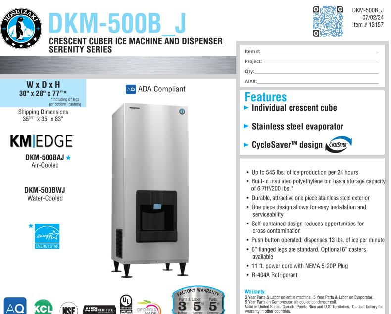
\*Rated in accordance with AHRI Standard 820(I-P). Capacity based on 100% of total volume x 30 lb/ft<sup>3</sup> average density of ice.
