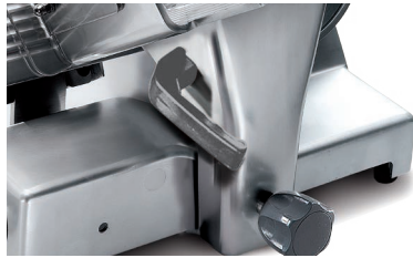
The carriage is quickly removable without tools.
