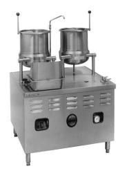
Steam generator will be automatically filled with hot water and brought to 15 PSI (1kg/cm²) pressure when heat and water switches are turned on and automatically drained under pressure when switches are turned off. Cold water condenser will automatically condense exhausted steam into water before releasing it to drain. Unit also includes safety valve, low water cut-off, water strainer, and descaler.
