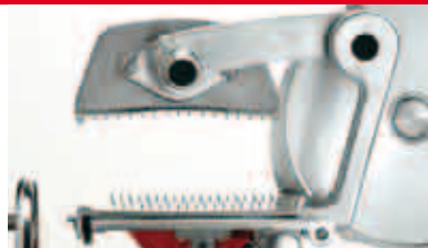
Lateral movement with a clamping arm to slide product through
