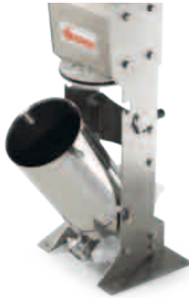
Product loading without removing cylinder
