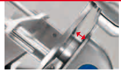
Increased gap between blade and machine body
