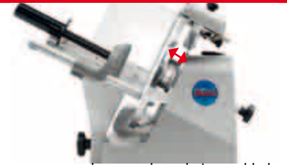
Increased gap between blade and machine body
